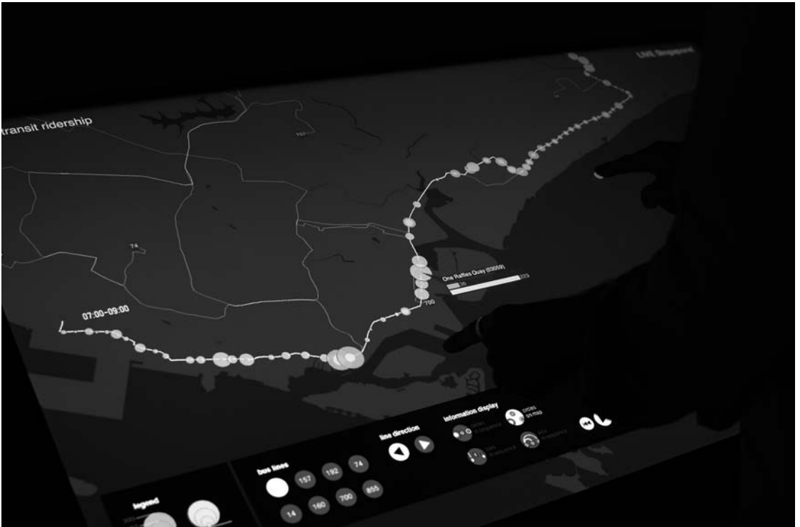
Figure 5. Touching Transport . Interaction : Zoom and pan the map; move in time; select time range (aggregate data); switch views (different perspectives); select bus line + direction (filter data); details on demand (filter data). Visualization : Glyphs showing boarding and alighting pax per station; glyphs on a map showing spatio-temporal relations (cluster, areas); time-series with glyphs showing spatio-temporal relations (at a glance); arc diagram showing flow of pax (OD, clusters); histogram showing pax over time. Task : Presenting knowns: revealing unknowns: personally relevant insights. Audience : Public: laypeople and experts.
