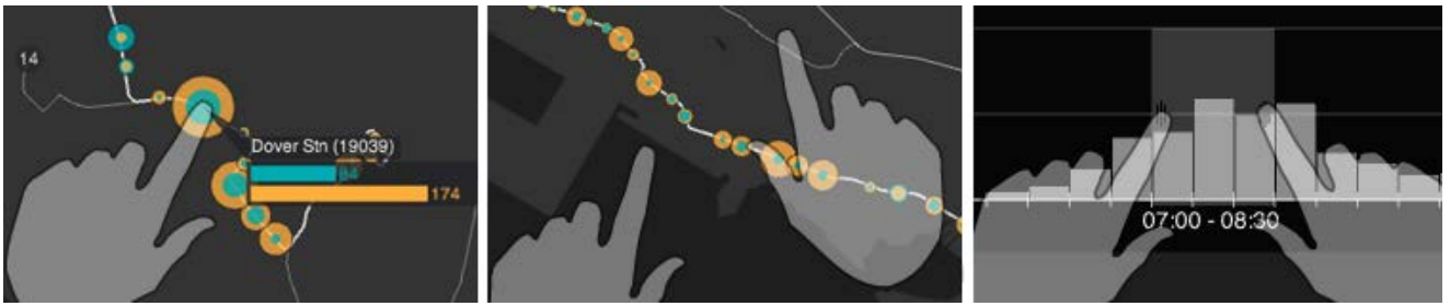
Figure 2: (a) Tap to select a bus stop, (b) free-form map manipulation, and (c) dual finger time range adaptation.
