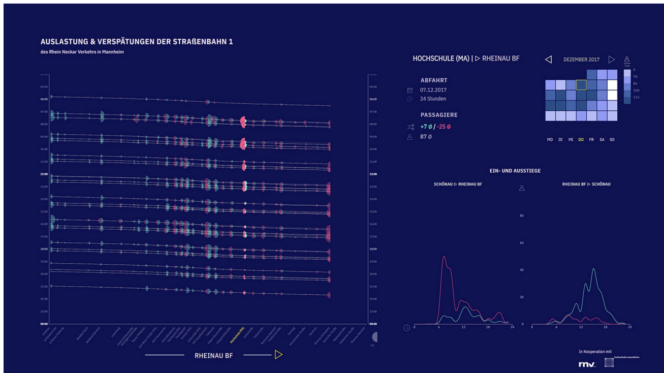
Fig. 4 Visualizes passenger flows as well as time plan and delay data in an extended Marey chart (left). On the lower right, boarding and deboarding passenger counts are displayed as two line charts for both directions
