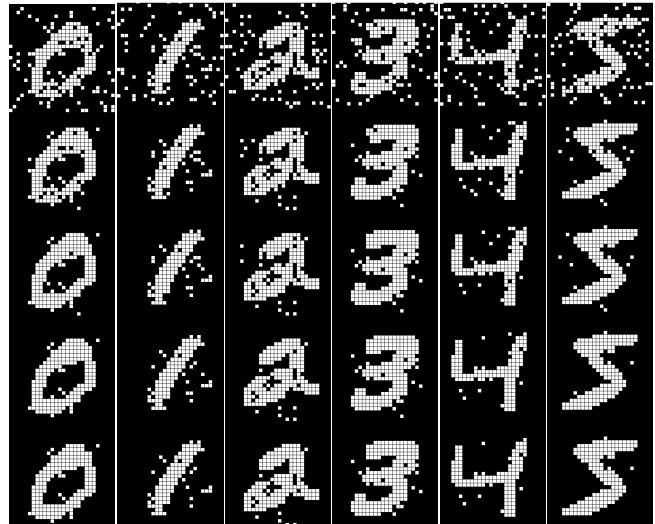
Fig. 4. After training, we start with a noisy 28 \times 28 pixel image, where 100 pixel at a random position are inverted. The images below are computed using the Euler-method with a time step size of 0.1 in 25 iterations. Only on each 5-th iteration an image is presented.
